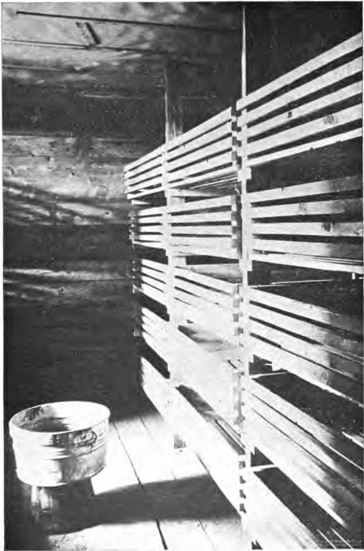
Fig. 45. Interior of disinfecting chamber, showing slat-work bins and position of tub used for a gas generator.
